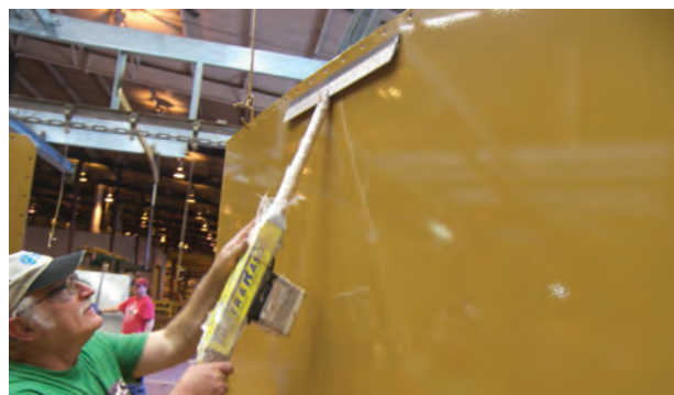
QC specialist running an 1100 volt holiday tester over 100% of coated tank panels.
