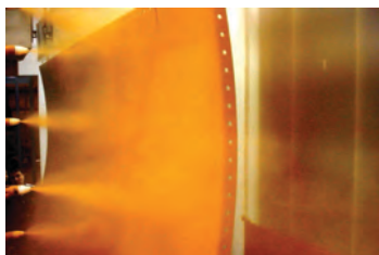
Laser eye directed powder-coat spray nozzles.
