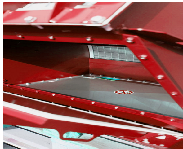
View of Inspection Door on R-IQR
